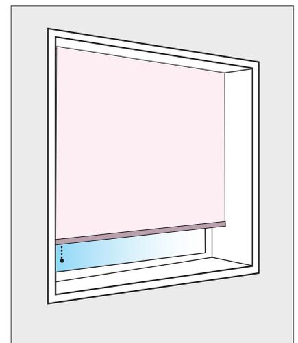
**RECESS FIT** is where the blind will sit inside of the window frame.
