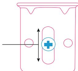
Bracket needs to be fixed with the longer edge to the wall or architrave (as per this image).
