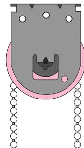
Ensure the tongue on the control bracket sits inside groove of the chain winder all the way
